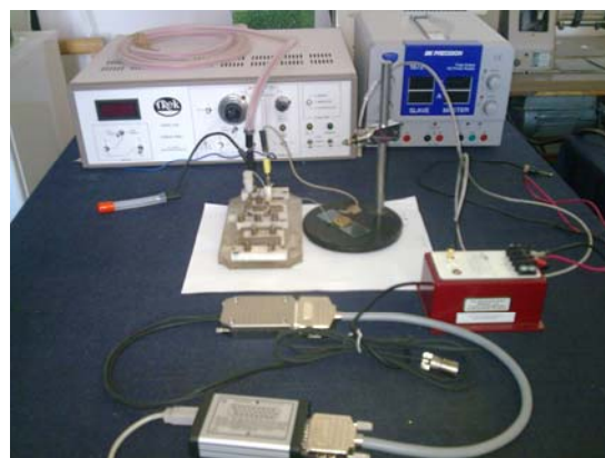
Fig. 2. Experimental setup for field-induced thickness strain measurements.
