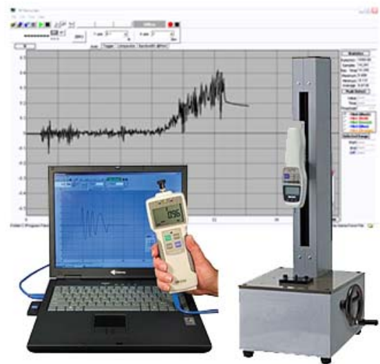
Fig. 5. Imada stand, digital gauges and recorder screenshot. Adjustable ramp is not shown.
